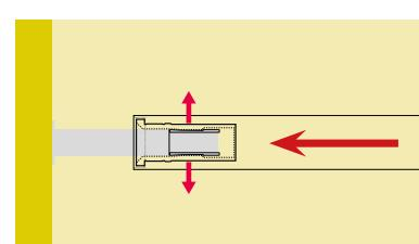
Push the shelf over the bracket. The plug will expand and the shelf is firmly fixed.
